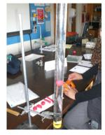
This session was spent looking at turbulence and laminar flow. We experimented with water and plasticine as to how different shapes fall – an introduction to streamlining.
